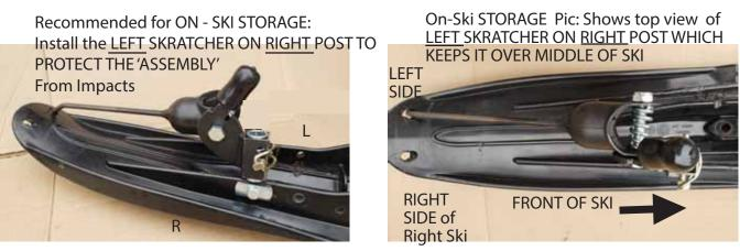
Raised 'Collar' on oval post bolt washer faces RIB and post bolt must be Extremely Tightened until washer is MAKE SURE 5/16" fully tight Nut is and stays against EXREMELY ski rib TIGHT!
