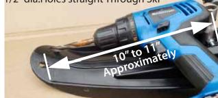
Then ANGLE your DRILL - LIKE THIS - APTER THE INITIAL HOLES ARE MADE - TO FIT TIPS THRU Easily.
