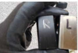
Scratcher Bracket SOUARE TUBES ARE MARKED: L - LEFT R - RIGHT Stamped into Steel
